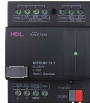
M/FCU01.10.1 module are combine FCU control and floor heating control, it has High-Medium-Low Fan Speed and also cooling and heating control if selected FCU function in ETS , it has 7 channels floor heating control if selected by ETS, Support 7 digital temperature sensors.
