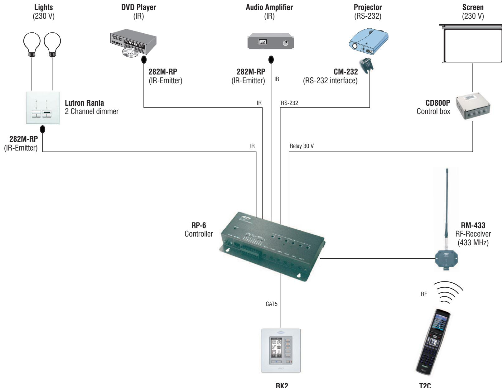
The RP-6 is a control processor and the heart of this control system. It provides IR, RS-232 and relais control ports for all devices in the home cinema. The RP6 has a connection port for RTI inwall control panels (e.g. RK2) and for the RF antenna (RM-433), which can be addressed by any RTI handheld control panel (e.g. T2C). All system commands and device status are stored on the RP-6. This ensures the secure and comfortable control of the system with two independent control panels.
