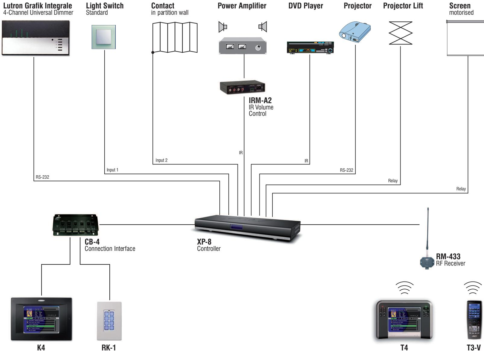
The XP-8 is a high-end remote control processor for automating the operation of electronic systems in homes and office buildings. The combination of a blazing fast MPU, real-time/multitasking operating system, and tremendous expandability make the XP-8 the perfect solution for large-scale and complex projects.
